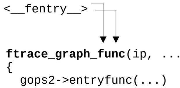
The diagram shows a call to `<__fentry__>` in the code block. Two arrows branch from the `<__fentry__>` label: one points down to `ftrace_graph_func(ip, ... { gops2->entryfunc(...)` and the other points down to `gops2->entryfunc(...)`.
